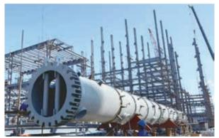
5. Large scale turbine hub of the first 12MW wind power equipment in the world
